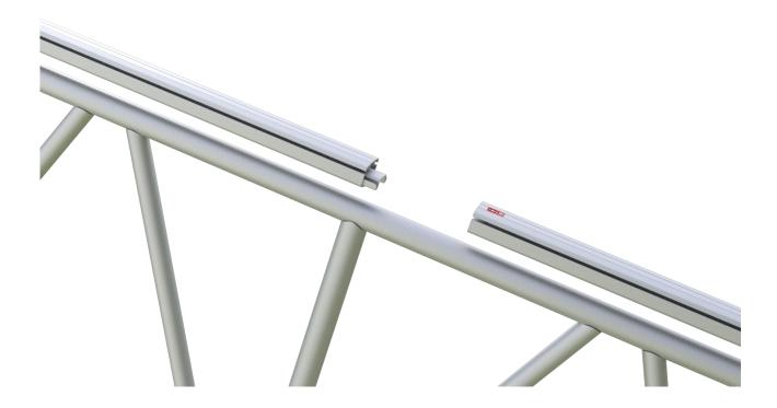
Install the UA0035 alloy track spigot half way into the existing DeepFlow $^{\text{TM}}$  tracking. Secure in place by tightening the handwheel against the bottom of the tracking.
