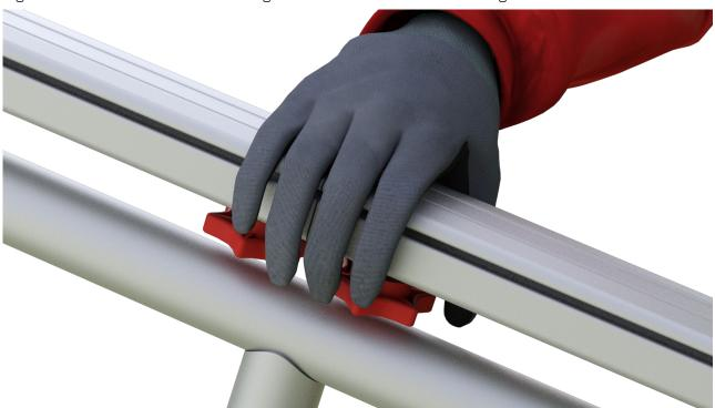
If using a track compressor, attach the spigotless US0001 end piece to finish off the tracking and terminate the tracking with a DESSA track compressor.
