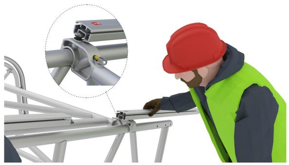
Install the UA0035 alloy track spigot half way into the existing DeepFlow  $^{\text{TM}}$  tracking. Secure in place by tightening the handwheel against the bottom of the tracking.
