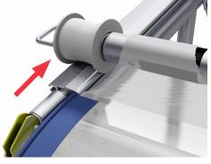
2.0 Ensure sheet pulling wheel and keder engage with the sheet track. Manually feed sheet through track for first 300mm.
