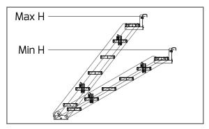
Note: the above table relates to application range when using tube connector brackets RB0011 and RB0012 only. The height measurement is taken to the centre of the scaffold tube to which the connector bracket engages.
