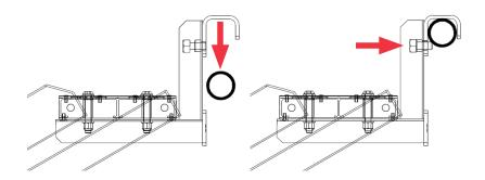
Use brackets RB0011 and RB0012 to attach the DESSA RANGER™ Stair to 48.3mm scaffold tubes. The brackets can be secured to the tube using the integrated bolt fixing, thereby preventing uplift.
