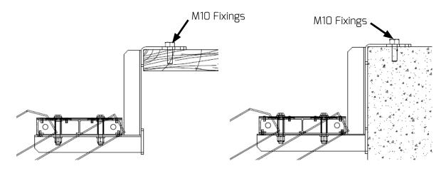
For horizontal surfaces use brackets RB0021 and RB0022 with M10 fixings to secure.
