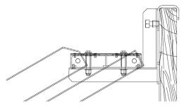
The RB0011 and RB0012 brackets are also to be used with timber joists up to 50mm in width. The anti-uplift bolt can be used to secure the stair by tightening lightly ito the timber joist.
