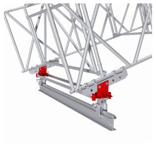
2) Used in conjunction with 0.7m bearer (UA0011) and anti-uplift castor (AA0002) to provide mobile support to an 18 degree duo-pitch roof. Used with Plettac ledgers to create an assembly of castors working in tandem in line with roof beam lines.
