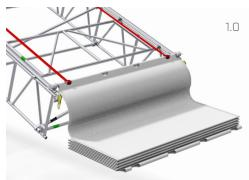
1.0 Fix 2no. DESSA pulling straps or ropes to sheet tensioning bar at outer two pocket locations. Offer sheet to roof bay.
