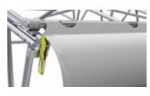
4) Connect rope to sheet tensioning bar and offer assembly to beam line, aligning wheel and sheet keder to the sheet track.
